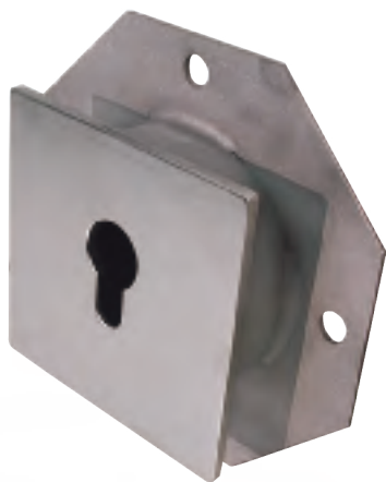
Wall Anchor Face plate 95x95 mm, back plate 140x140 mm, depth 34 mm. Stainless steel*. To be bolted onto the pool wall 14152 Wall Anchor
