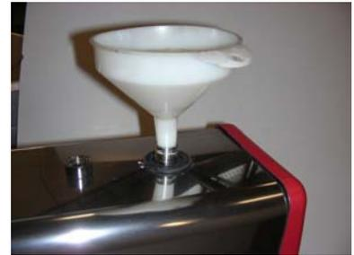
Citric acid deliming agent is odourless and harmless and it does not harm the steam generator's components. If other type of deliming agent is used, bathing during decalcification is not allowed.
